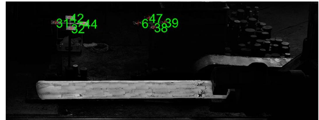
Target system during forging measurement (Hurník et al., 2021)
