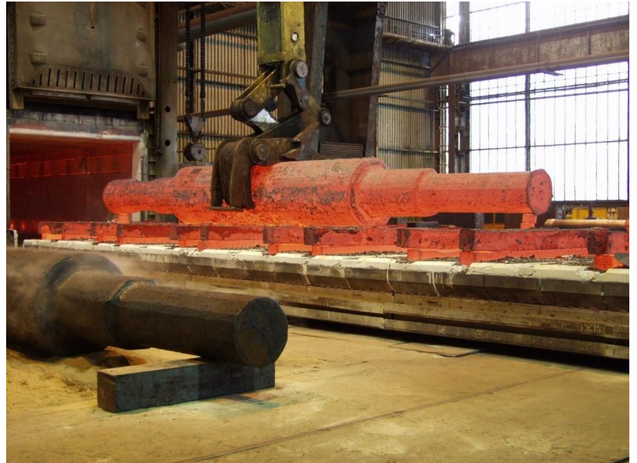
Heavy forging (simufact.com)
